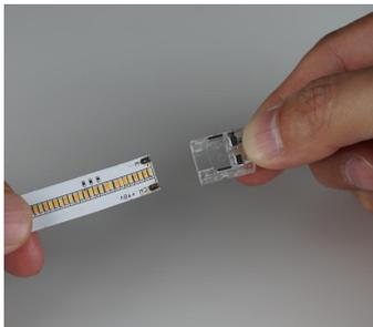
Insert one end of led strip and wire connector into both ends of the connection terminal respectively to ensure that the metal clip is on the same side as the metal solder pad of led strip.
