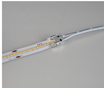
Meanwhile make sure both ends are closely connected, Press the metal clip down with the appropriate plier to ensure that the metal clip is inserted into the appropriate position ,and connection completed.
