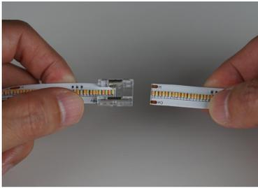
Insert each ends of led strips into the end of the connection terminal respectively, make sure the metal clip is on the same side as the metal solder pad of led strip.
